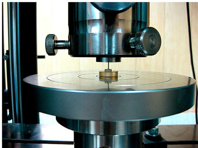
**Figure 1.** A cylindrical stainless steel plunger attached to the load cell of the universal testing machine loading on MTA inside a root section.
