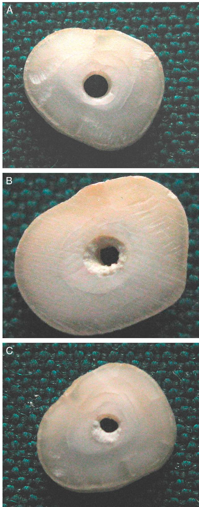
**Figure 2.** Various failure modes. (A) Adhesive failure; note the clean canal wall. (B) Cohesive failure within MTA. (C) Mixed failure; note the MTA residual inside the canal.
